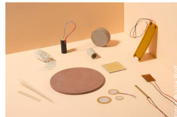
Three different groups of shape-changing materials: dielectric elastomers, piezoceramics, shape-memory alloys
