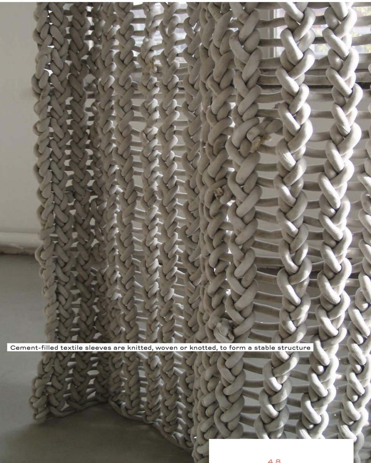
Cement-filled textile sleeves are knitted, woven or knotted, to form a stable structure
