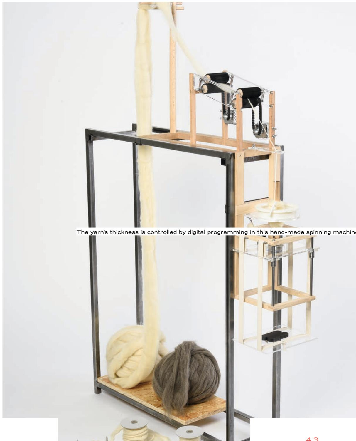
The yarn's thickness is controlled by digital programming in this hand-made spinning machine
