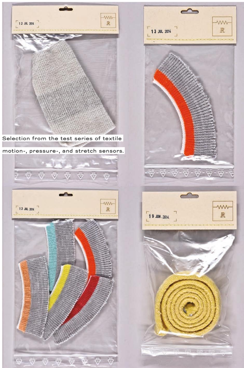
Selection from the test series of textile motion-, pressure-, and stretch sensors.
