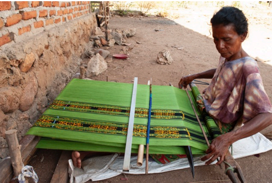
54) A stake loom with circular warp in Baranusa on Pantar Island; east of Alor ~2010 -2015. No reed is used! © Christopher D. Buckley
