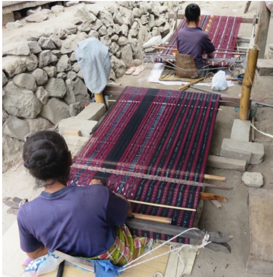
26) Two of several types of body-tensioned ground looms, in use by Palu'e weavers. Photo: Stefan Danerek /Osi Kula 2021.
