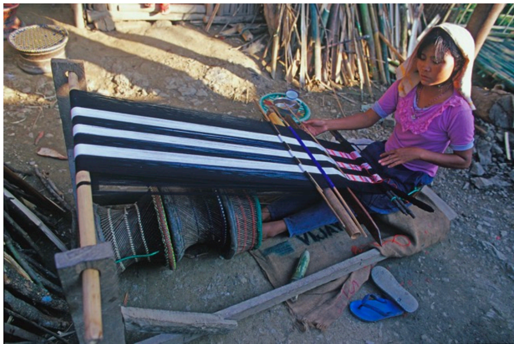
79) A station loom in Nagaland, NE-India. Date & photographer unknown. Notice the segmented foot rest, realized from several drum stools lined up. Material of choice changed, but the expression of segmentation remains - in Nagaland and on Flores. Buckley Archive
