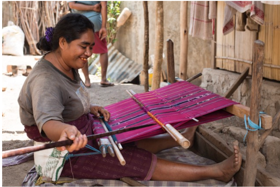
30) Weaver in Atadei-region on Lembata; forked branches are used as warp posts. ~2010-2015. © Christopher D. Buckley
